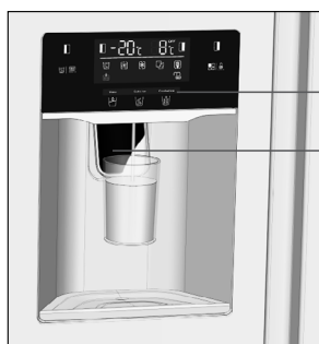
Cubed ice, crushed ice, cooling water mode Paddle switch
